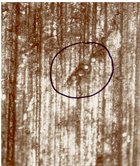
Figure 2: Piston ring surface with cat fines trapped in graphite flakes magnification 280:1
